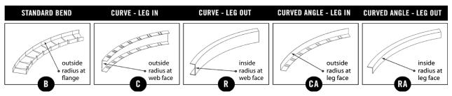
WIDTHS: Up to 12" LENGTHS: Up to 35' + GAUGES: 22, 20, 18, 16, 14 MATERIAL: c-studs / joist, track, angle (I-metal), furring (hat) channel, channel (CRC) sections
