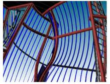
Radius Track Corporation designed each unique framing assembly for the office and rehearsal spaces where Ninety-four percent of the curved framing members fabricated are one-of-a-kind including the knife edges.
