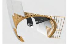
The Radius Track Design Team used Rhino 3D modeling software to design the 218 unique pairs of steel stud and track panels for the framing of the hull's exterior surface.
