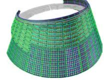
Designed and modeled in 3D prior to fabrication, the unitized panels and adjacent systems were analyzed for clash detection and fit.
