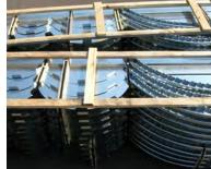
Radius Track® used 3D modeling to design the curved CFS framing solution for each size of the convex shape, fabricated the pieces needed, labeled them, and shipped them to the site ready to be installed.
